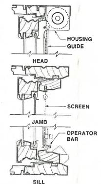
EGRESS WINDOWS — 2436CC, 2440CC, 2448CC, 2460CC and 2468CC (units designated with single asterisk in size chart) are available with sill-mounted roto operator and special hardware, to function as egress windows to comply with codes requiring openable area of not less than 5.7 ft² (0.53 m²) and no dimensions less than 22" (559 mm) wide and 24" (610 mm) high. Units are to be installed with sill not more than 44" (1 118 mm) above the floor.
