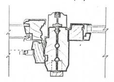
FIXED UNITS (CASEMENT AND AWNING)—both vent-size and fixed-size—are shown in section at right with Pella double glazing at head, welded insulating glass at jamb and %" (15 mm) insulating glass at sill. Fixed units will accept glass to 1" (25 mm) thick.
